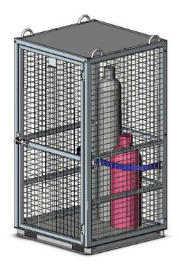
The type MGBC Gas Cylinder Storage Cage has been designed primarily as a secure storage unit for building sites and mines. The lockable gate, mesh sides and roof sheeting ensure cylinder and gear security. The Cage is fitted with a 4 point Crane lift and Forklift pockets underneath for transport. The internal load binder prevents cylinder movement during transport.
